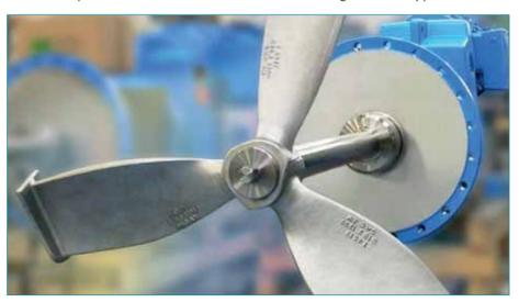
Agitators from MUT-Tschamber are used for a wide variety of applications. The main components of the assembly are the drive, the insertion shaft and the agitator element, as well as flanges, seals and bearings
