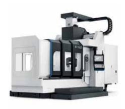
unparalleled flexibility for large-part machining. The spindle can be supplied with up to 90 or 120 HSK-A63 tools or 60 HSK-A100 tools, depending on the option selected by the customer.
