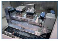
a 40-taper model, thanks to its dynamics. This is due to 2.2 g linear axis acceleration, 0.2 second spindle acceleration to 16,000 rpm, simultaneous tool changing, 0.7 second and repositioning of the spindle for the next cut and reduced machine downtime for tool replenishment thanks to the 40-station tool magazine. 14 or 22 tools are optional and the 2APC arrangement means that there is only a short delay before the first cut is taken on the next part.
