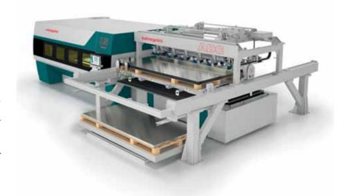
for sheet metal loading and unloading. Its strengths are compact footprint, rapid cycle times and fast installation. Like all the Salvagnini automations, ADC is also equipped with the new AVC adaptive vacuum control technology. AVC constantly monitors the vacuum degree in the gripping suction cups and vacuum generation is
