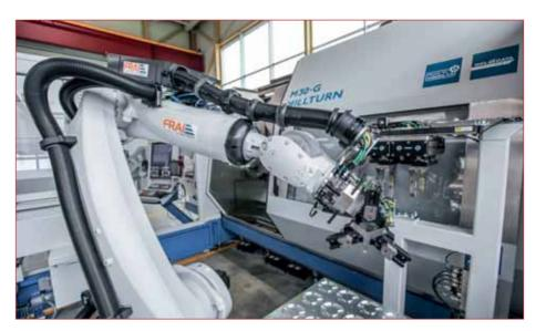
One of the most flexible automation versions of machine tools or processes is the articulated robot in a robot cell
