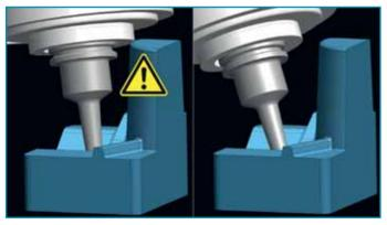
Potential collisions with the machine head are automatically avoided in 5-axis simultaneous avoidance milling
