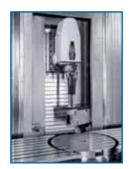
Tool change now takes place safely behind the work table, avoiding interference with fixtured workpieces and contributing to thermal stability
