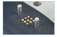
coupling of power supply in pallet pools, buffers and FMS systems is effortless. This means easier adaptation of automated workpiece loading in these systems.
