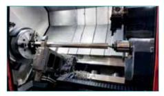
The benchmark shaft on the SMEC 4500 LM. The machine is equipped with a main spindle, NC-controlled steady rest and tailstock and a 12-station turret (with four stations for driven tools) and is ideally suited for shaft machining up to approximately 3 m in length
